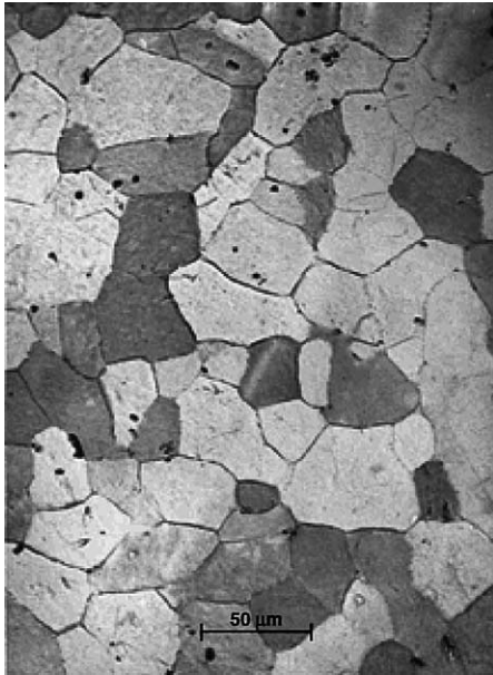
Fig. 4. Photomicrograph of nominal-purity as-cast delta Pu with a grain size of 40 \mu\text{m} [11].
